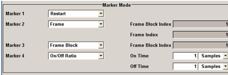
The **Marker Mode** section is where the marker signals at the MARKER output connectors are configured.
