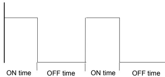
The ON time and OFF time are each expressed as a number of symbols and are set in an input field which opens when ON/OFF ratio is selected.
