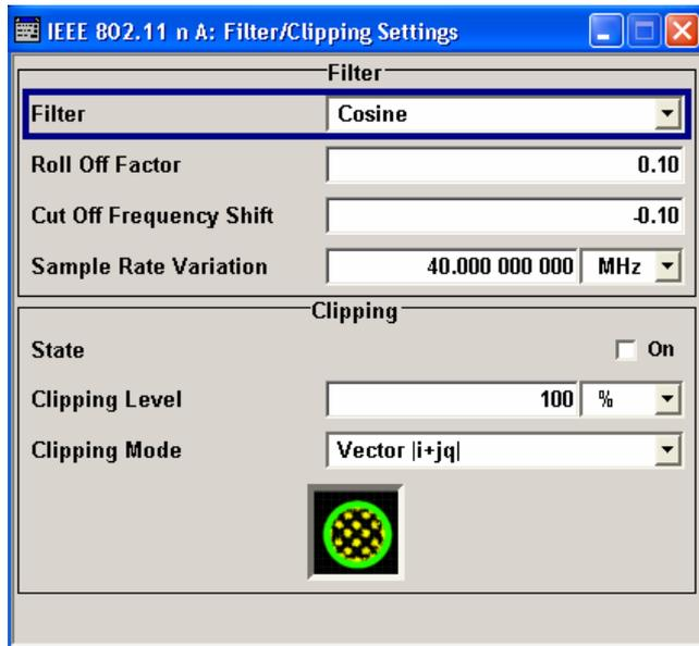
In the **Filter** section, the settings are made for the baseband filter.
