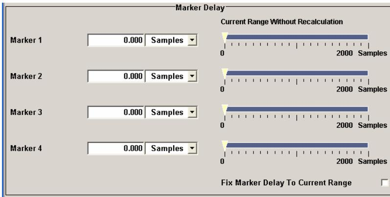
The **Marker Delay** section is where a marker signal delay can be defined, either without restriction or restricted to the dynamic section, i.e., the section in which it is possible to make settings without restarting signal and marker generation.
