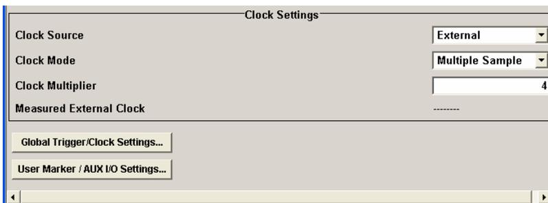
The **Clock Settings** section is where the clock source is selected and - in the case of an external source - the clock type.
