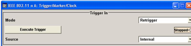
The **Trigger In** section is where the trigger for the IEEE 802.11n WLAN-N signal is set. Various parameters will be provided for the settings, depending on which trigger source - internal or external - is selected. The current status of signal generation (**Running** or **Stopped**) is indicated for all trigger modes.
